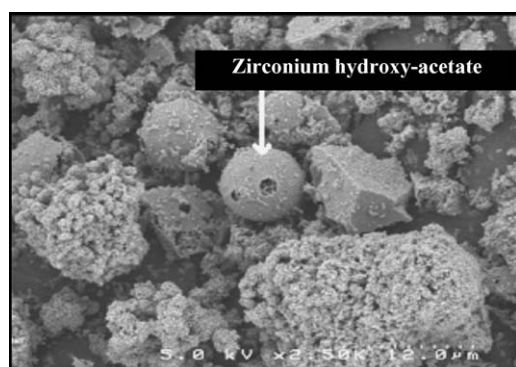
Fig. 4. FESEM micrograph of the YSZ powder synthesized with 10% nitric acid, revealing the presence of unreacted zirconium hydroxyacetate precursor.
